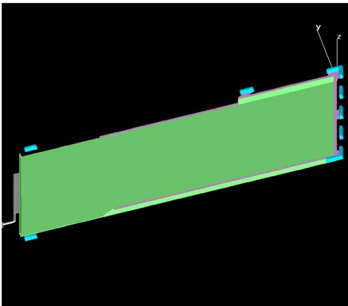
Part, gate, reservoirs and flash geometry assembled in the same reference system
