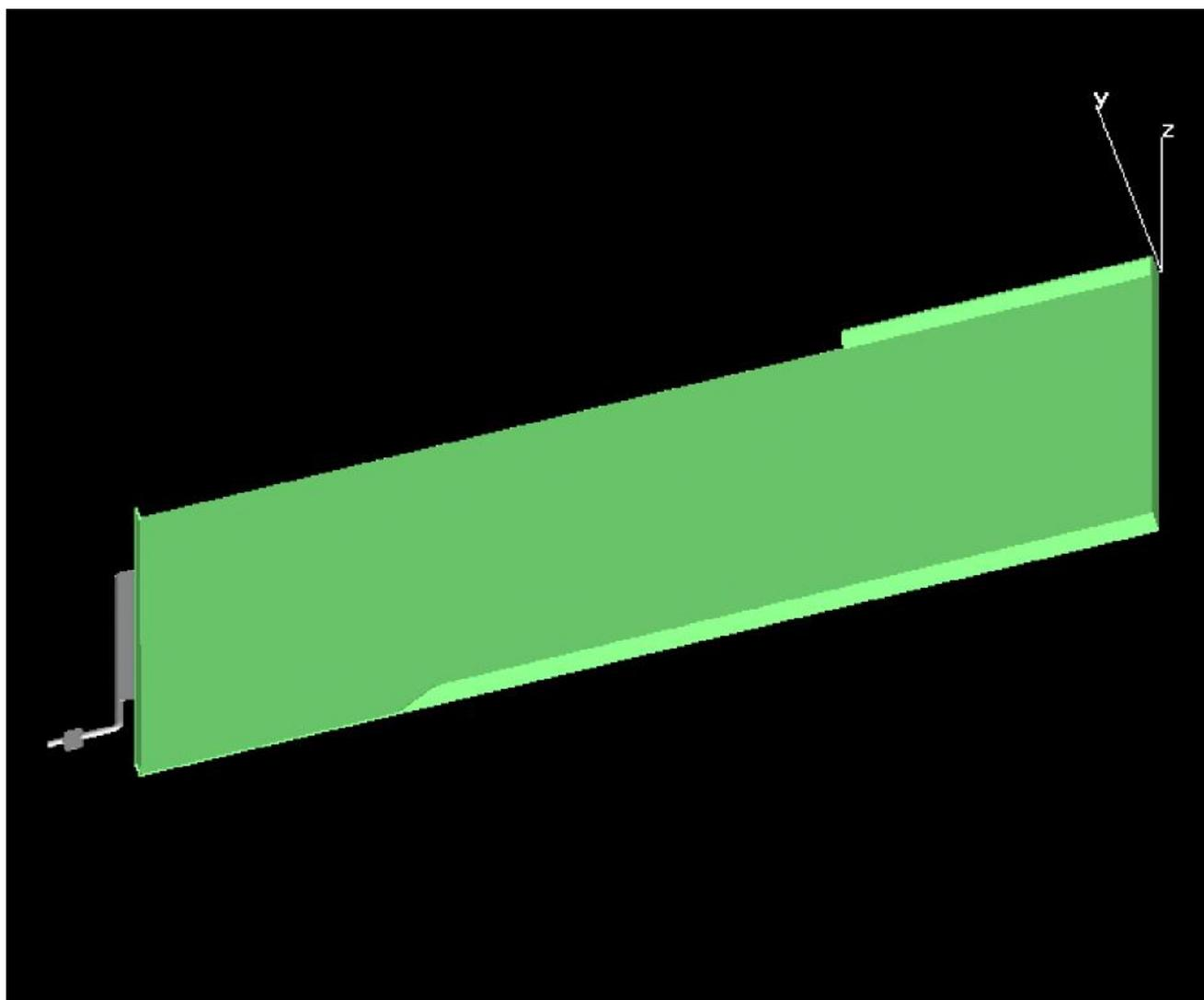
Part geometry and gate geometry assembled in the same reference system
