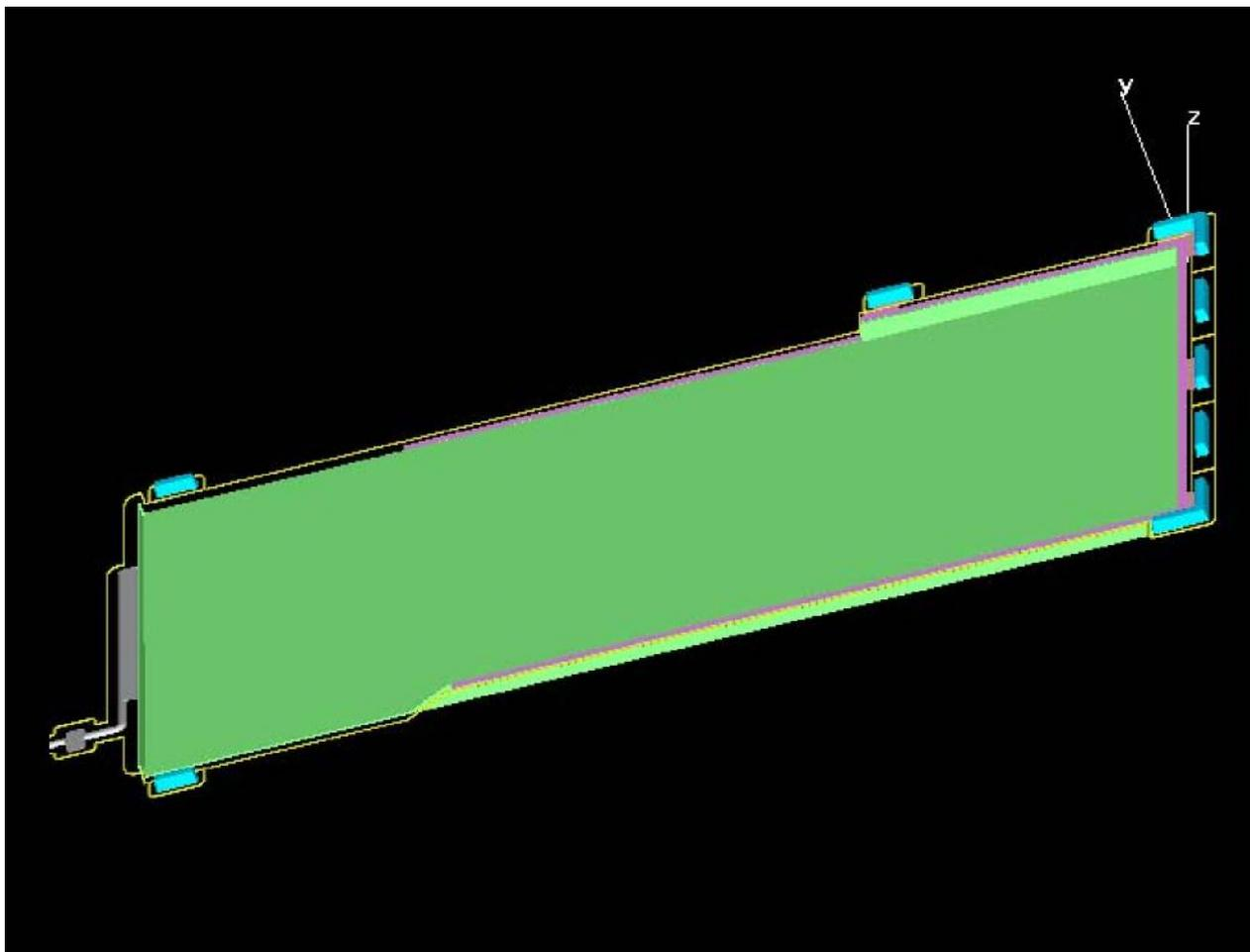
Part, gate and reservoirs, flash and gasket geometry assembled in the same reference system
