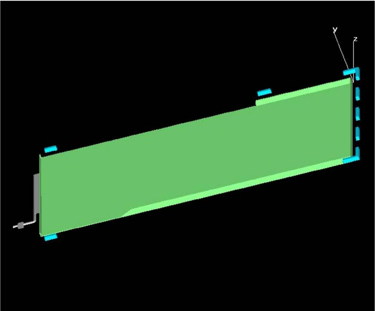
Part, gate and reservoirs geometry assembled in the same reference system
